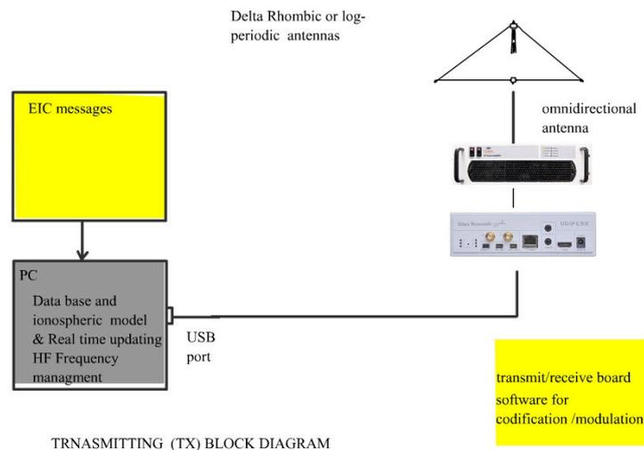
**Figure 5** Example of block diagram of a single TX HF point of the HF network.
