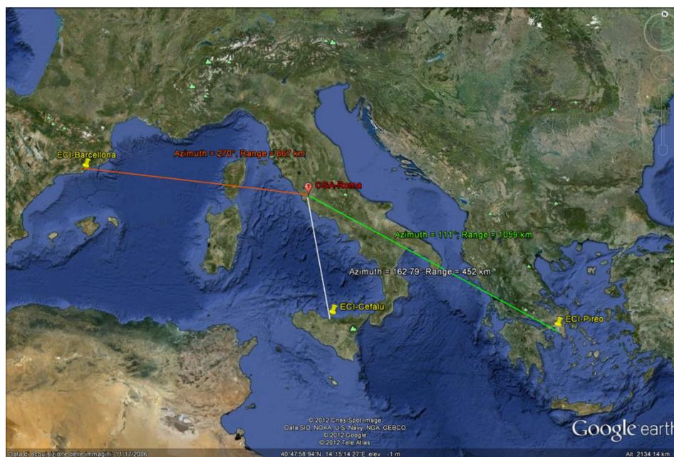
**Figure 1** Reference scenario and radio link connection among ECIs and CGAs
